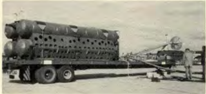
Palletized rig, easily loaded in any C-130, uses engine bleed air to atomize water as it leaves nozzles, controls flow and volume.
