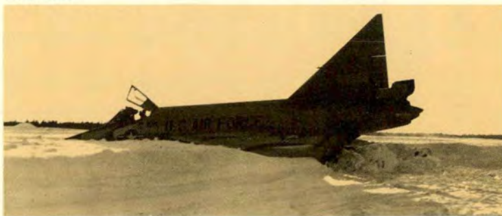
Snow on the runway—obscures visibility, defeats braking, compounds steering, covers markings, hides the turnoffs. Beware!
