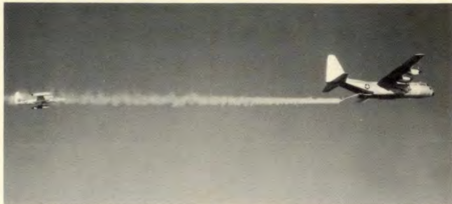
Special water - tanker C-130 creates artificial icing cloud during low - speed tests evaluating aircraft and engine anti - ice systems.
